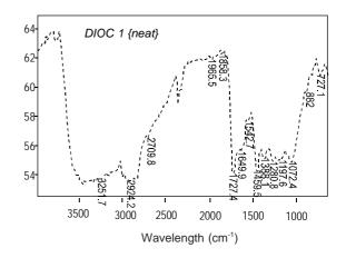
Fig. 1. Spectrum of infrared spectroscopy of *Dioclea reflexa* oil.
