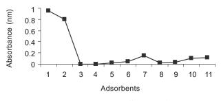
1: Treatment; 2: untreated effluent; 3: ferrous chloride; 4: calcium hydroxide; 5: imp orient 20 PWG; 6: imp orient A-100; 7: imp orient WWT-50; 8: coal ash 1(untreated); 9: coal ash 2(1st regenerated); 10: coal ash 3(2nd regenerated); 11: coal ash 4(3rd regenerated).
