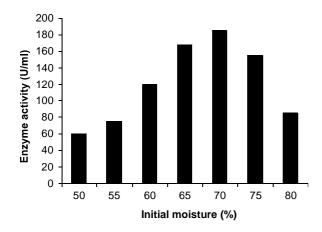
**Fig. 2.** Effect of initial moisture content of medium on the production of  $\alpha$ -amylase by *B. subtilis*-239.
