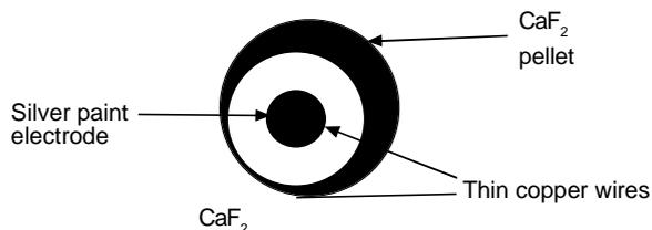
**Fig 5.** CaF<sub>2</sub> pressed pellet with silver electrodes used for the measurement of dielectric constant.
