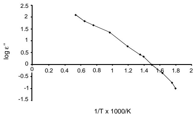
**Fig 3.** Plot of imaginary part of dielectric constant against inverse of temperature 1/T for  $\text{CaF}_2$  (Pellet).
