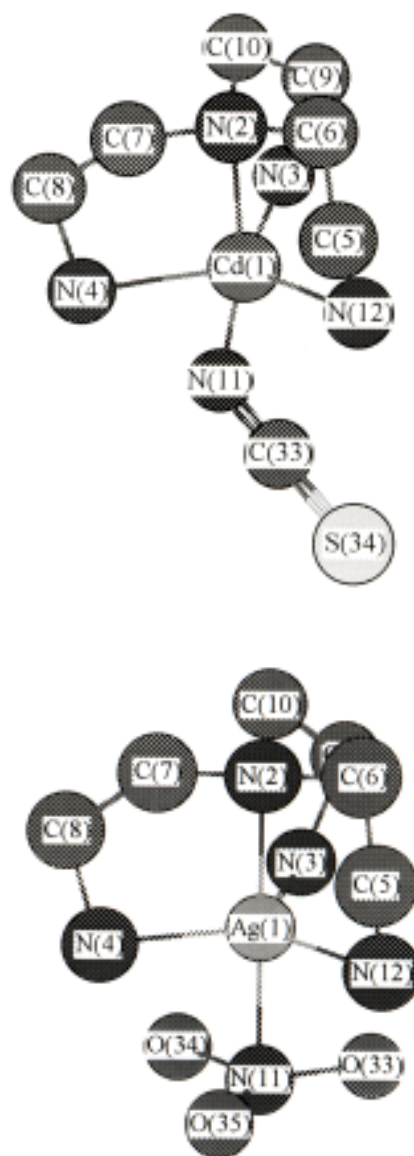
Fig 2(a). Slightly distorted trigonal bipyramidal coordination environment around Cd-atom (b) Spherically symmetric tbp coordination environment around Ag-atom.
