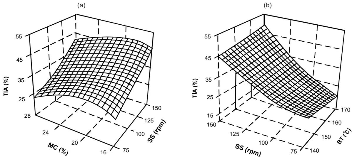
**Fig 1.** Effect of (a) Moisture Content (MC) and Screw Speed (SS) and (b) Screw Speed (SS) and Barrel Temperature (BT), on Trypsin-Inhibitor Activity (TIA).
