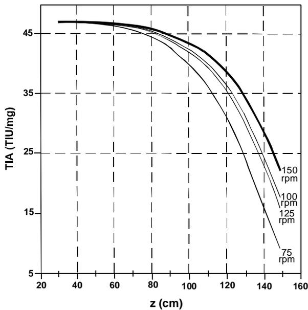
Fig 3. Inactivation of Trypsin Inhibitor (TI) along the Screw Channel ( $z$ ) at 20% Moisture Content and 150°C Barrel Temperature and 75,100, 125 and 150 rpm Screw speeds.
