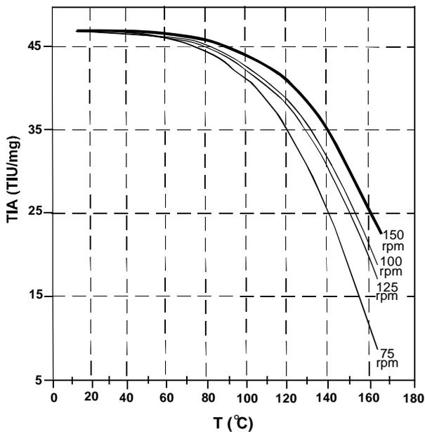
Fig 4. Inactivation of Trypsin Inhibitor (TI) with increasing Soybean Temperature ( $T$ ) at 20% Moisture content, 150°C Barrel Temperature and 75,100,125 and 150 rpm Screw speeds.
