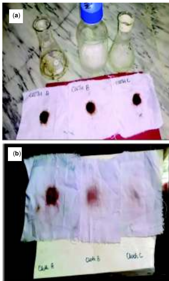
Fig. 5. Cloth A was dipped in water only, cloth B was dipped in detergent solution only, cloth C was dipped in detergent and amylase solution (a) stained cloths before treatments (b) stained clothes after treatment.
