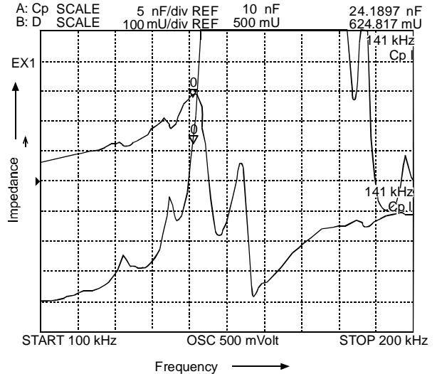
**Fig. 3.** Value of capacitance after thirty five shocked w.r.t frequency (100 kHz-200 kHz); capacitance in nF at frequency of maximum impedance when shocked from 150 °C - 20 °C.
