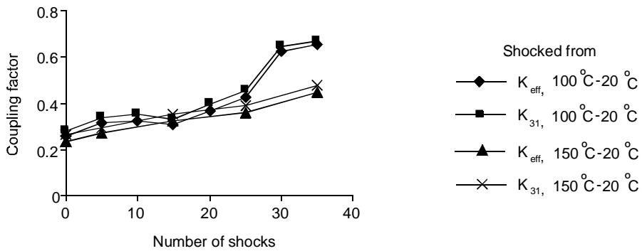
**Fig. 5.** Change in coupling factor ( $K_{31}$ ,  $K_{eff}$ ) against number of shocks from 100 °C - 20 °C and from 150 °C - 20 °C in deionized water.
