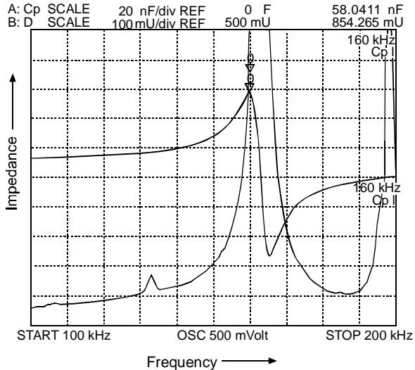
**Fig. 1.** Value of capacitance for un-shocked disc w.r.t frequency (100 kHz-200 kHz); capacitance in nF at frequency of maximum impedance.
