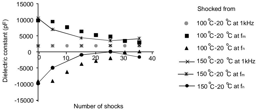
**Fig. 4.** Change in dielectric constant against number of shocks, at frequency 1kHz and frequencies of maximum and minimum impedance.
