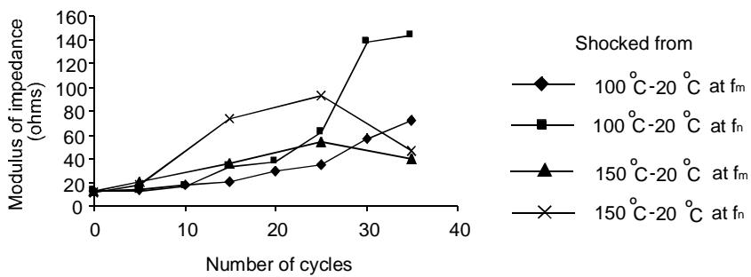
**Fig. 6.** Change in modulus of impedance ( $|Z|$ ) against number of shocks from 100 °C - 20 °C and from 150 °C - 20 °C in deionized water.
