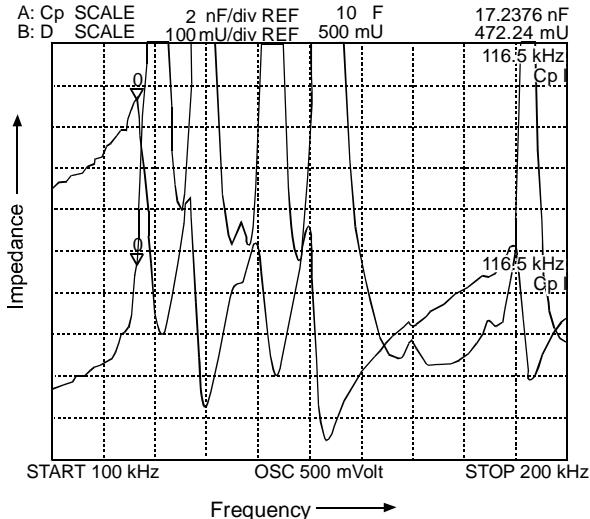
**Fig. 2.** Value of capacitance after thirty five shocks w.r.t frequency (100 kHz-200 kHz); capacitance in nF at frequency of maximum impedance when shocked from 100 °C - 20 °C.
