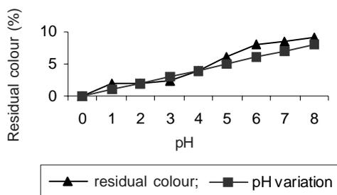
Fig. 3. Residual colour with variations in pH.
