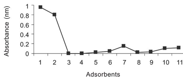
1: Treatment; 2: untreated effluent; 3: ferrous chloride; 4: calcium hydroxide; 5: imp orient 20 PWG; 6: imp orient A-100; 7: imp orient WWT-50; 8: coal ash 1(untreated); 9: coal ash 2(1st regenerated); 10: coal ash 3(2nd regenerated); 11: coal ash 4(3rd regenerated).
