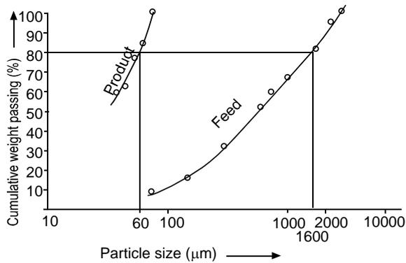
Fig. 8. Bond work index (Wi) of the phosphate rock.
