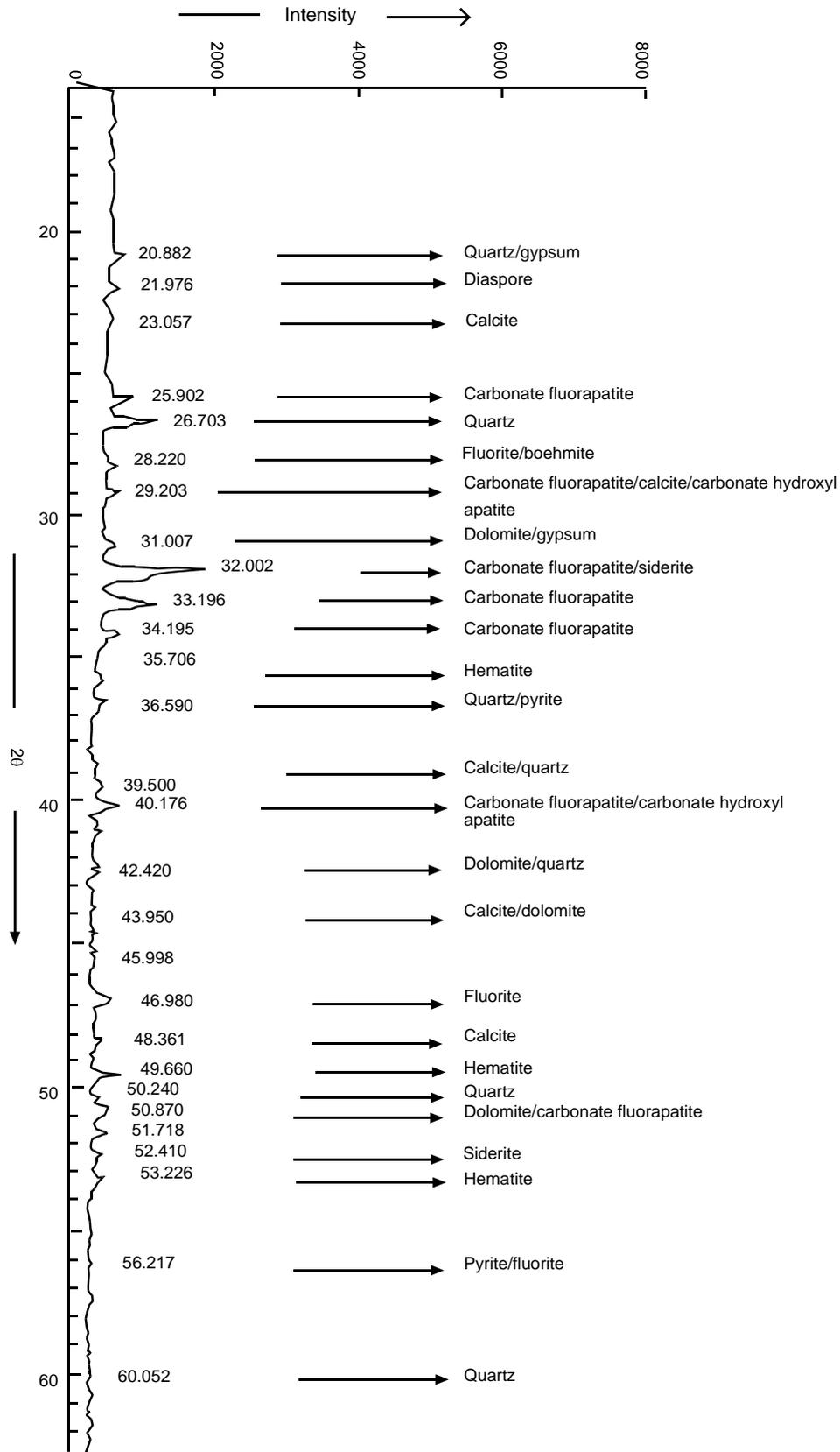
Fig. 7. X-ray diffractogram of Kakul (Hazara) phosphate rock.
