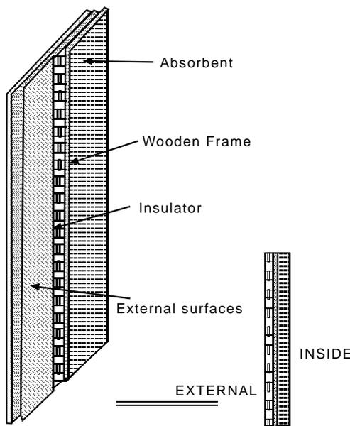
**Fig. 3.** Detailed structure of the main enclosure panel.
