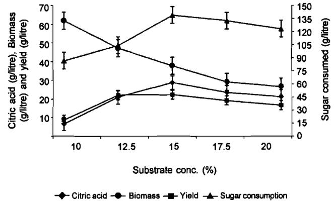
Fig. 1. Evolution of citric acid and biomass during the fermentation using different substrate concentration.
