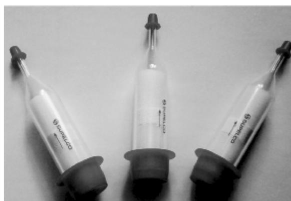
**Fig. 2.** PUF/XAD-2/PUF cartridges.
